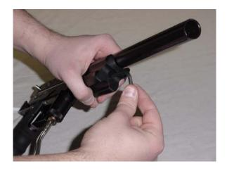
As a quick tip – many people have found it easiest to adjust the velocity by fully turning the velocity screw into the marker and then adjusting it out until the velocity is up to speed.
