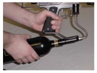
For monthly lubrication remove the upper Bolt and the Hammer Assembly (see the Quick start for assembly instructions). Lubricate the Sear and the Trigger thru the lower chamber and lubricate the Upper Bolt and the Hammer Assembly.
