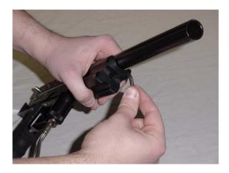
When changing the velocity of your AM-P Illusion be sure to fire several shots to make sure that the setting is locked in. We have found the best performance of the AM-P Illusion is reached when the marker is firing at around 280 feet per second.
