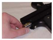
\*\*\*\* Note – The Upper bolt should always have two holes pointing downward and one pointing upward. If the upper bolt is upside down the marker will not be able to shoot.
